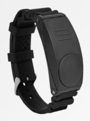
**Smart wristband** - a telemetry sensor placed on the driver's wrist, designed to receive information on the relative change in electrical resistance of the skin and transmit it digitally via radio to a receiver.
